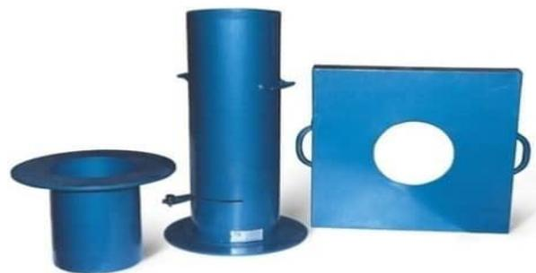
*Figure; Soil testing equipment by replacement method.*
