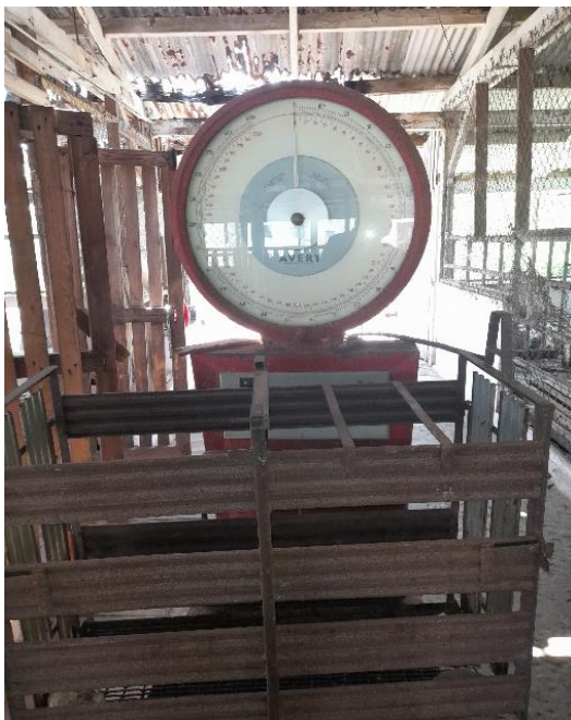
Fig 6: Picture showing the weigh equipment used at the Bodles Research Station to weigh the Goats monthly.
